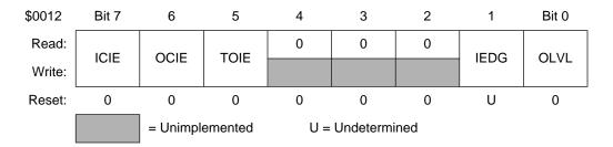
Figure 8-2. Timer Control Register (TCR)
