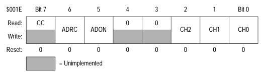
Figure 9-1. A/D Status and Control Register (ADSC)
