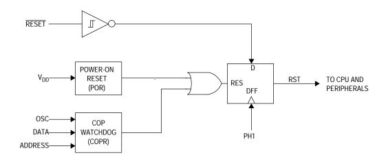
Figure 4-1. Reset Block Diagram
