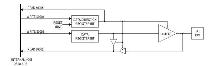
Figure 6-3. Port C I/O Circuitry
