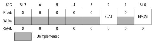
Figure 10-1. EPROM Programming Register (EPROG)
