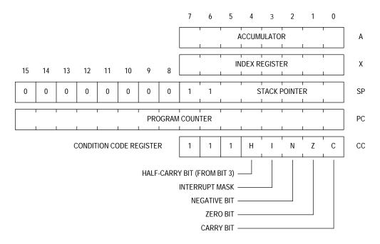
Figure 12-1. MC68HC05 Programming Model
