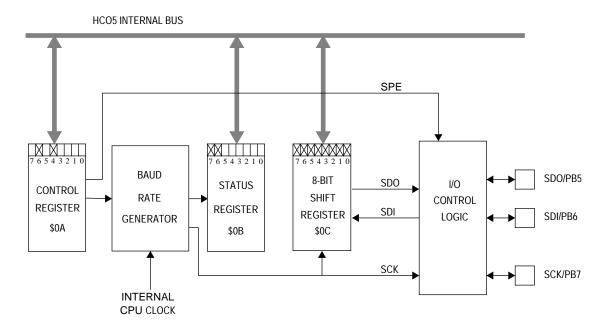
Figure 7-1. SIOP Block Diagram
