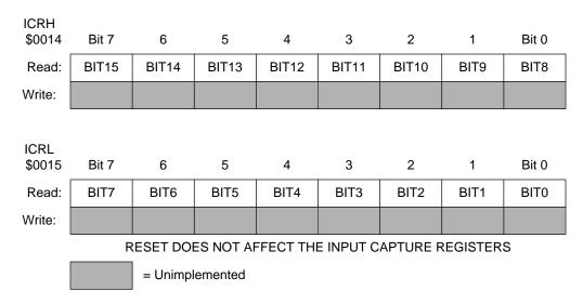
Figure 8-6. Input Capture Registers (ICRH and ICRL)
