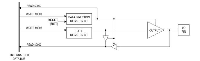
Figure 6-4. Port D I/O Circuitry
