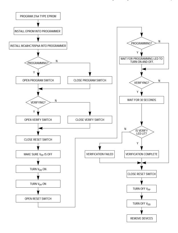
Figure 10-2. MC68HC705P6A EPROM Programming Flowchart
