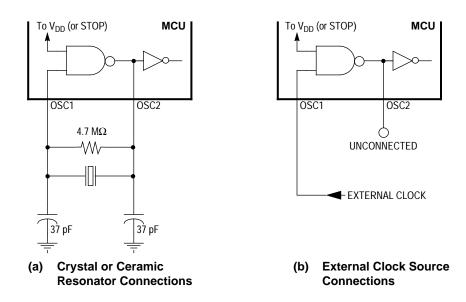
Figure 1-2. Oscillator Connections
