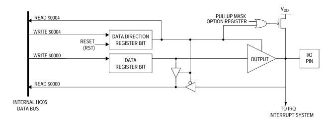
Figure 6-1. Port A I/O and Interrupt Circuitry
