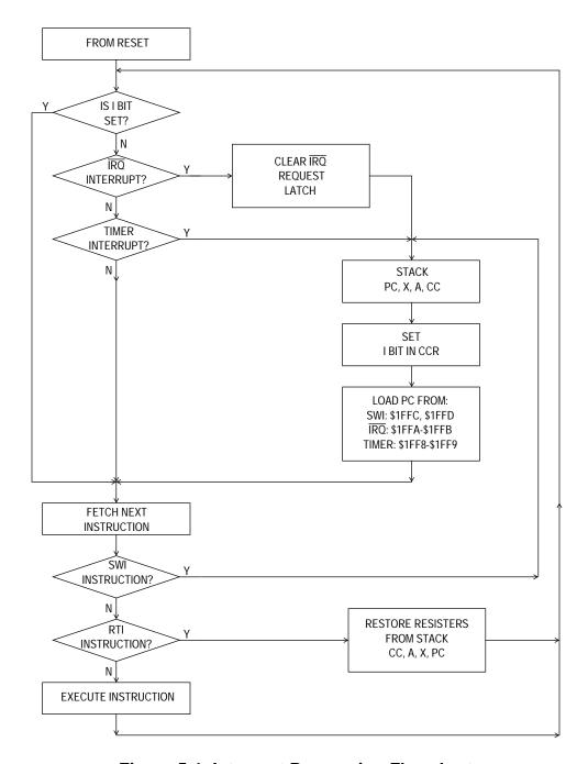
Figure 5-1. Interrupt Processing Flowchart
