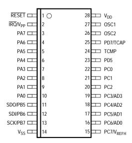
Figure 3-1. User Mode Pinout
