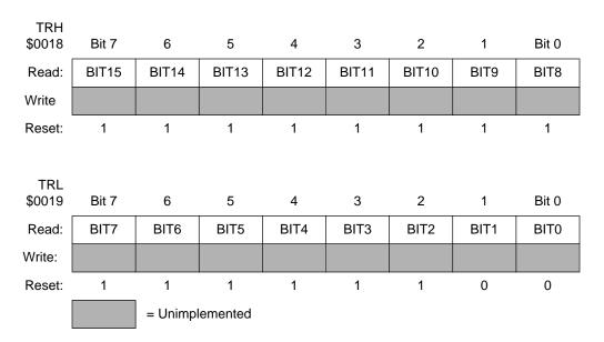
Figure 8-4. Timer Registers (TRH and TRL)
