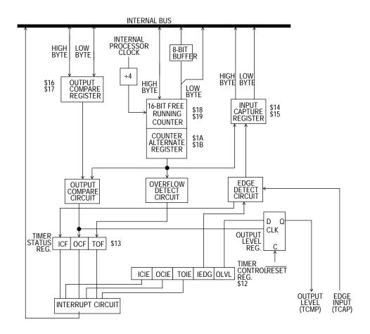
Figure 8-1. Capture/Compare Timer Block Diagram
