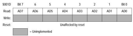
Figure 9-2. A/D Conversion Value Data Register (ADC)
