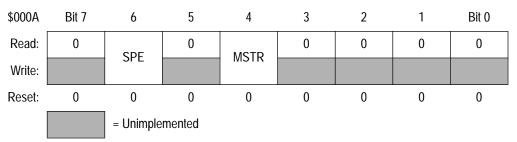
Figure 7-3. SIOP Control Register (SCR)
