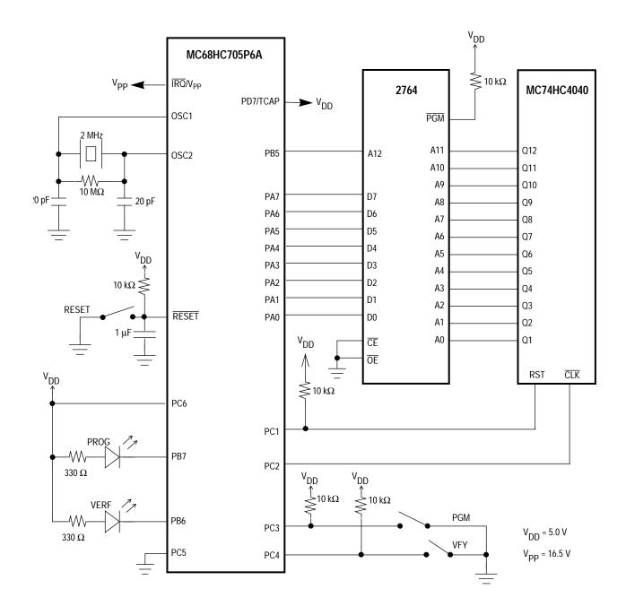
Figure 10-3. MC68HC705P6A EPROM Programming Schematic Diagram
