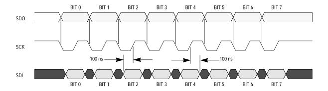
Figure 7-2. SIOP Timing Diagram
