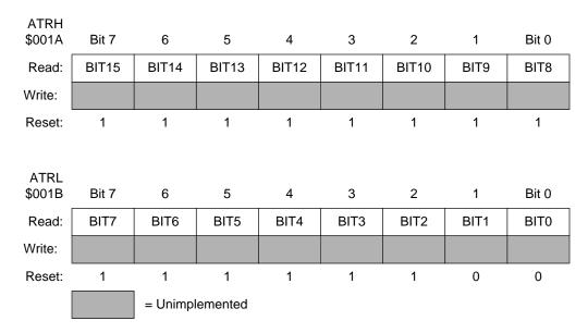
Figure 8-5. Alternate Timer Registers (ATRH and ATRL)
