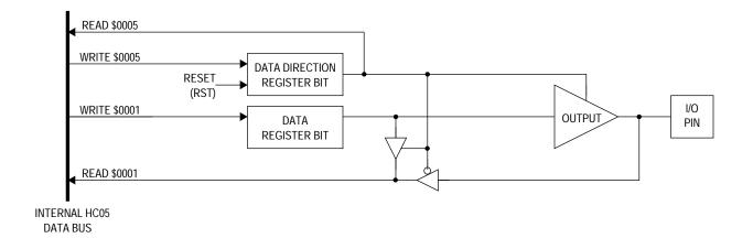
Figure 6-2. Port B I/O Circuitry
